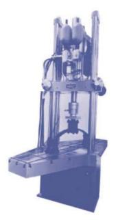
The need to perform endurance tests on heavy duty leaf springs led to an investment in a servohydraulic test system that would give servotest's customers great accuracy, repeatability and versatility.
