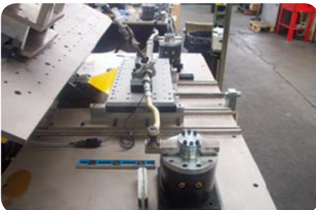
Two off Servotest Hydrostatic Linear actuators apply end loads via a bell crank mechanism mounted on two large bearings housed under bed plate. The actuators are mounted under the tilting table to optimise customer space requirements for the test rig.
